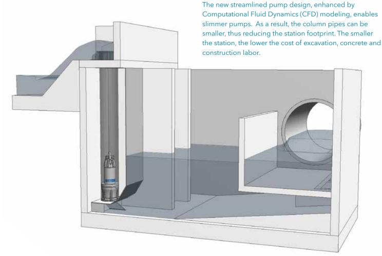
Because the pump station is a complex system, it is important to consider every aspect in the station design. Pump system reliability and efficiency depend not only on the performance of the
