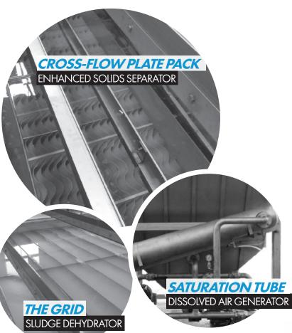
FRC's PCL dissolved air flotation system is a high-built solid/liquid separator designed for high flow rates and low hydraulic surface loading rates. The combination of **The Grid** and **Cross-Flow Plate Pack** create sludge with high dry solids content. The air dissolving **Saturation Tube** ensures only the finest bubbles are introduced into the flotation cell.
