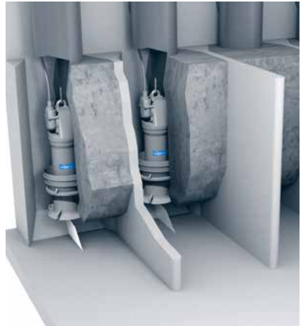
Pump station with formed suction intake in concrete.
